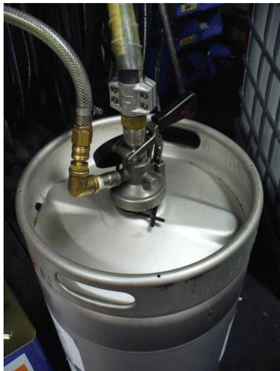
Filling Pentanes with Macro Valve Fill-head
