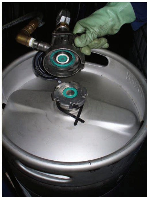
Macro Valve Fill-head: On disconnection there is no product residue on the Macro Valve and Coupler
