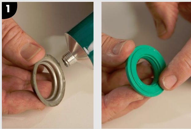
Lubricate spring retainer and profile seal with silicon lubricant.
