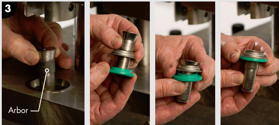
Remove the arbor from the base of #740-906 Valve Assembly Tool.
