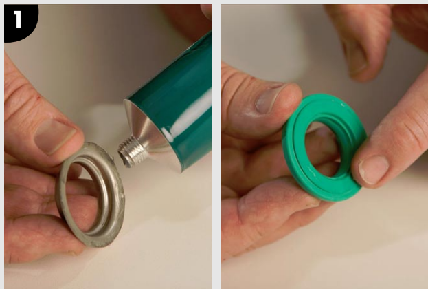
Lubricate the spring retainer and profile seal with silicon lubricant.
