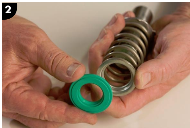
Using a new spring, spring retainer and profile seal, create the tube assembly.
