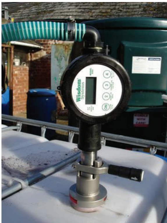
ADS Coupler with flow-meter mounted on CDS plastic valve
