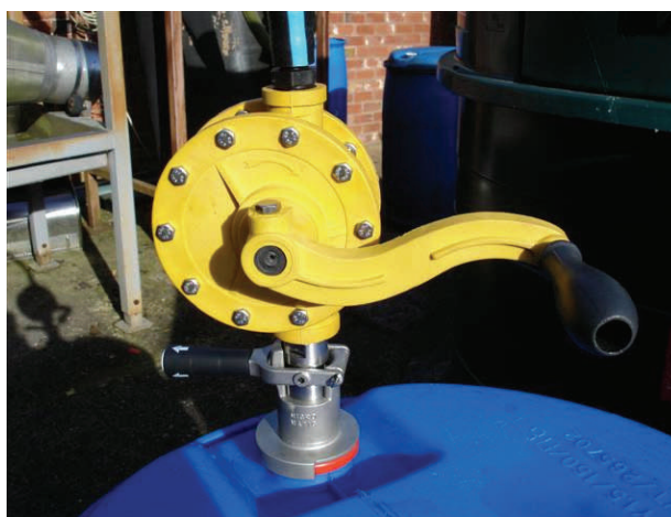
ADS Coupler with rotary manual pump mounted on CDS plastic valve
